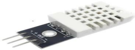
Fig Humidity sensor
