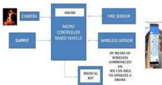
Fig.3.1 Block diagram of Fire Fighting Drone
