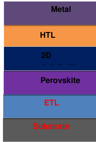
Fig.1.Schematic diagram of 2D-MOF Perovskite thin film.
