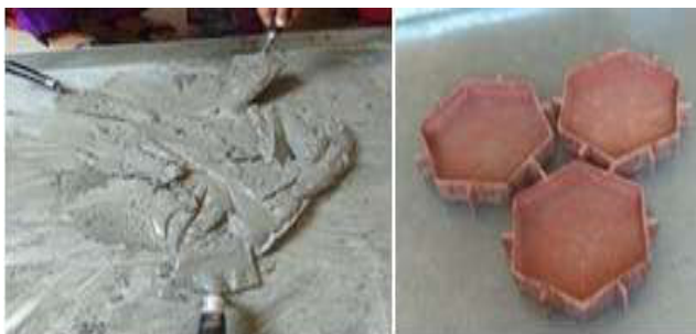
Fig. 2. Mixing and Mould for Paver Blocks
