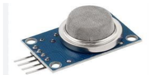
Fig Gas sensor
